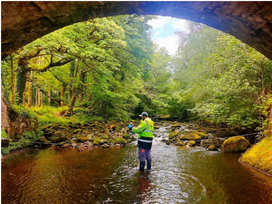
Figure 35 CDM Smith measuring discharge at Cladagh Bridge by dividing the channel up into sections.
