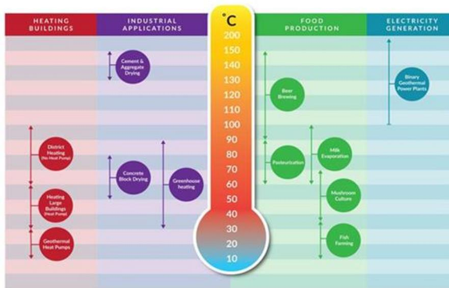
Figure 2. Applications of geothermal energy in Ireland.
