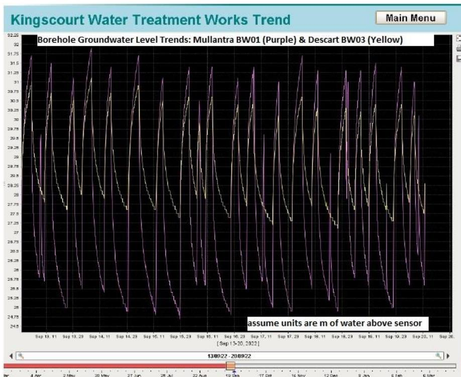
Figure 19: Scada Abstraction and Groundwater Level Data, September 2022.
