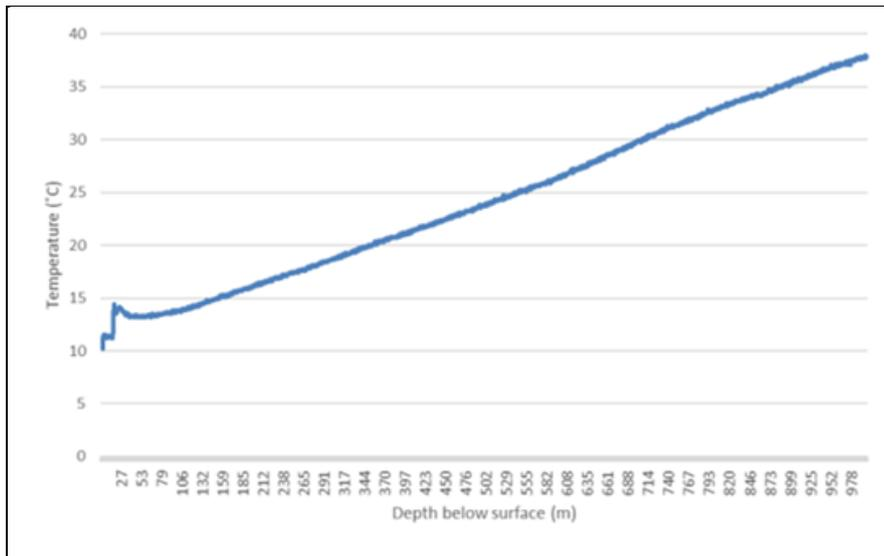
Figure 4. Fibre optic temperature profile obtained from Grangegorman geothermal borehole.
