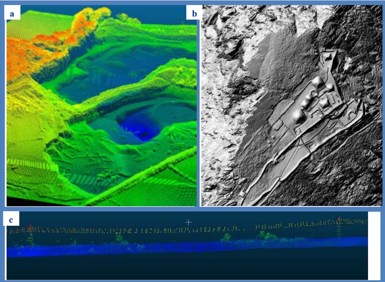
Figure 29 Example of LiDAR data from the Open Topographic Data Viewer a) Point data at a quarry site. b) Digital Surface Model of the Beehive huts on Skeillig Michael. c) Point data of Power line network
