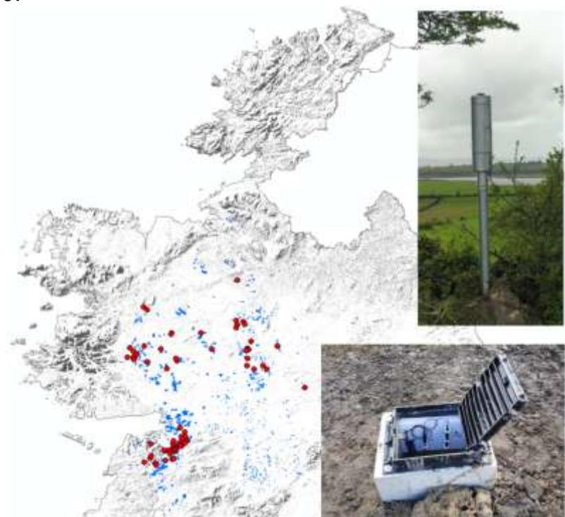
Figure 11: GW Flood Turlough Monitoring Network (red) overlaid on groundwater flood hazard sites (blue) (Mott MacDonald, 2010). Insets: permanent turlough water level monitoring equipment.
