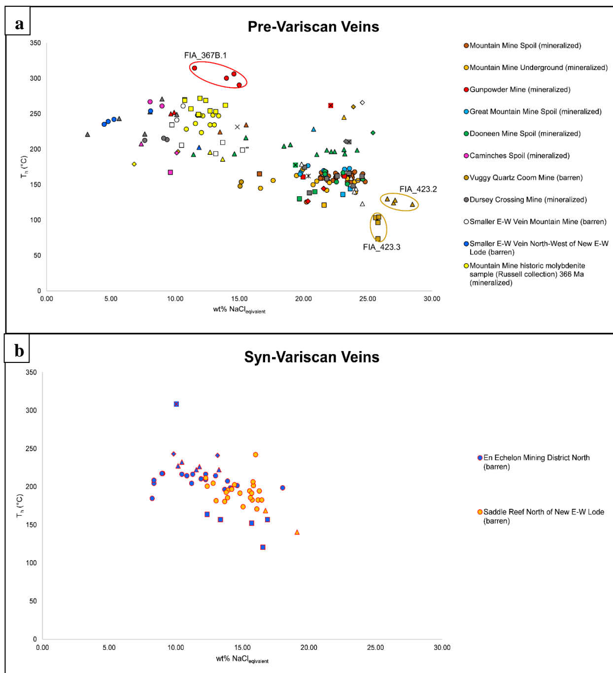
Fig. 2. Fluid inclusions from samples of the Allihies Plot of the salinity wt% \text{NaCl}_{\text{equiv}} versus the homogenisation temperatures T_h (°C). The different colours show the various locations, and the symbols indicate the individual fluid inclusion assemblages (FIA) within one sample.
