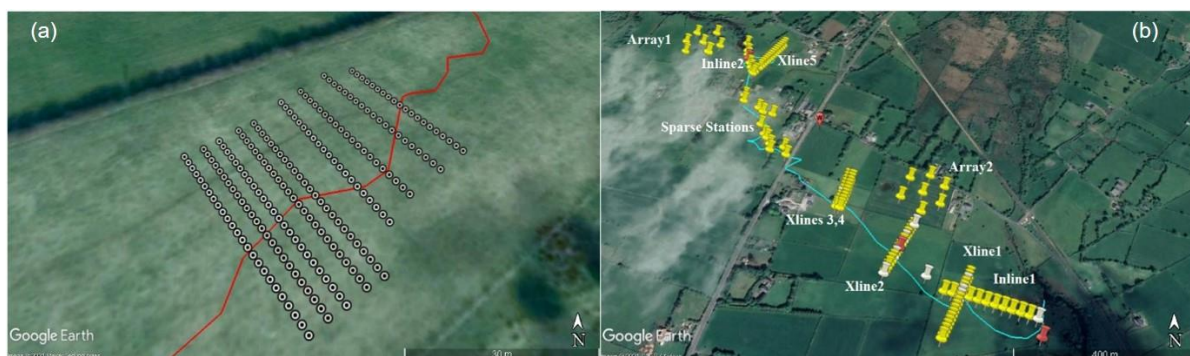
Figure 4. (a) The coverage of the 50*50 m 2 study area using moving linear profiles of 1Hz short-period seismometers, 15-20 th Dec. 2020, Pollnagran Cave, French Park, Co. Roscommon. (b) Seismic experiment between 29-30 th March 2021, Polltoophill-Poldeelin Cave, Gort, Co. Galway. For this experiment, we deployed several linear profiles to passively locate the conduit based on the Amplitude Location Method (ALM) as well as two seismic arrays each consisting of 7 stations to track the propagating wavefront generated by the Airgun shots at the Poldeelin Rising. It should be noted that here, because of the scale of the experiment, we mainly use 5Hz geophones, which are easier to deploy but less sensitive than the 1Hz seismometers used in the Roscommon experiment.
