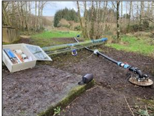
Figure 4: Pumping test rig setup on a former production borehole
