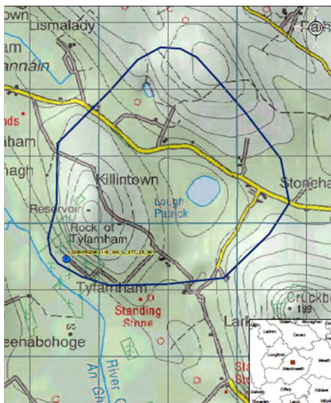
Figure 2: Multyfarnham GWS County Westmeath Groundwater ZOC
