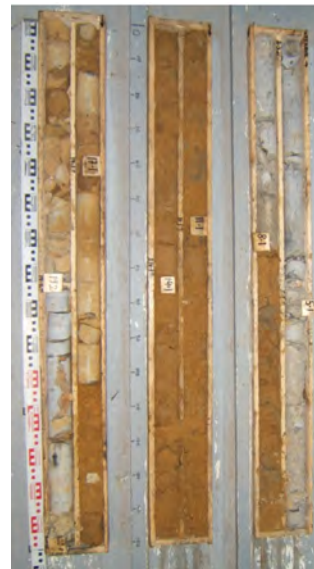
Figure 4a: Contoured Bouguer Anomaly values in microgals with a photo of core from a borehole in a gravity low (magenta) showing limestone with cavities filled with silty sand (8.1 – 18.8 m bgl).
