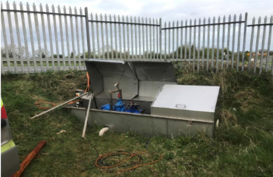
Figure 3.3 Arden Borehole 2 with logging tripod setup over borehole.
