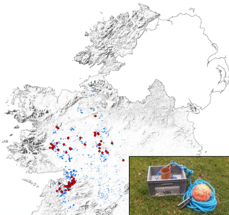
**Figure 2: GW Flood Turlough Monitoring Network (red) overlaid on groundwater flood hazard sites (blue) (Mott MacDonald, 2010). Inset: exploratory network monitoring equipment.**
