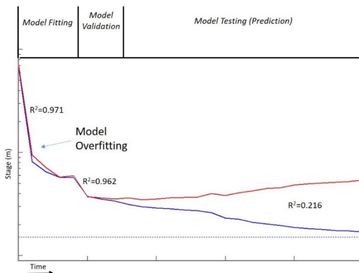
**Figure 5 – Demonstration of overfitting in a mathematical whilst attempting to calibrate a model for turlough stage with a small dataset**
