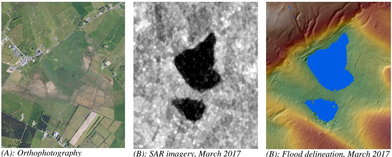
**Figure 4: Imagery of Castleplunket Turlough Co. Roscommon showing orthophotography of it empty (A), pre-processed SAR imagery of it flooded (B) and a flood delineation overlaid on LiDAR data (C)**
