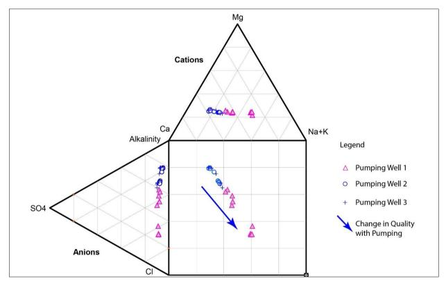
Figure 82: Durov plot illustrating changes in major ion content with pumping as additional saltwater was induced into pumping wells.
