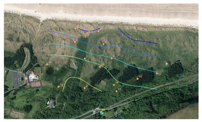
Figure 67: Piezometer locations and groundwater flow map, Winter 2017.
