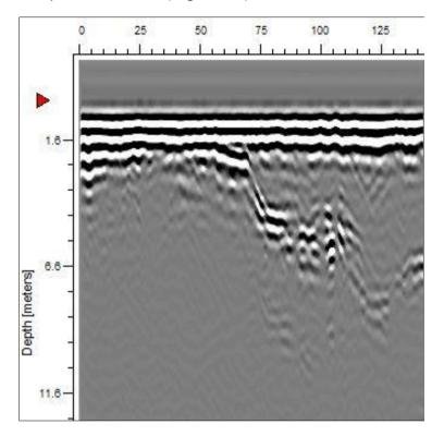
Figure 15: Ground Penetrating Radar profile, Colin Burn, Co. Antrim, reflecting the significant variations in peat thickness (up to 7m) across the catchment. Image: Alastair Ruffel, QUB.
