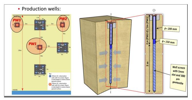
Figure 80: Pumping well design for the Magilligan Test Site. Wells PW2 and PW3 were pumped to intercept seaward-flowing fresh groundwater to enhance the possibility of drawing in salt water at PW-1. Well head water quality was measured with flow through cells at all three wells during pumping.
