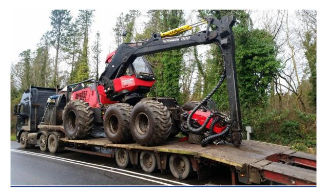
Figure 52: December 2017 - Toy delivery. Drenagh Sawmills Komatsu 931, 22 tonne harvester.
