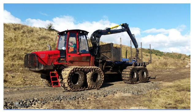
Figure 59: Drenagh sawmills Komatsu 865 8WD 19 tonne forwarder onsite, harvester off site after 15 day shift.
