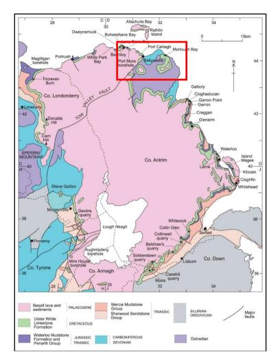
Figure 23: Simplified bedrock geology of the Antrim Plateau area showing distribution of the Cretaceous Ulster White Limestone Formation or 'Chalk' (adapted from Mitchell 2004). The NE County Antrim area of interest shown by red box.
