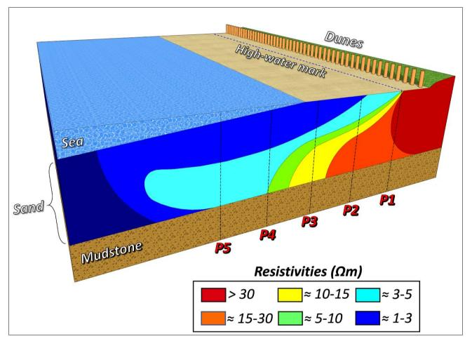
Figure 84: Revised conceptual model of saline intrusion at the Magilligan Test Site. In contrast to the classical basal wedge observed in more widespread studies, salt water induced into pumping wells derives from saline groundwater derived from the inter tidal recirculation cell, with high recharge rates generating an inverted freshwater wedge which extends below the low tide mark.
