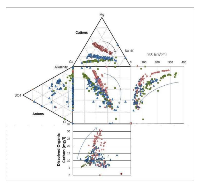
Figure 19: Expanded Durov plot summarising water quality in the streams draining the three test catchments. (Squares-Letterunshin, Circles-Garron, Triangles-Cuilcagh). Arrows reflect the evolution of water quality as flow increases, in which catchment waters with distinct base flow chemistries converge toward a common low SEC Na-CI water type.
