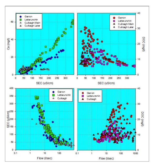
Figure 18: (Above) Plots of water chemistry with specific electrical conductivity (SEC) for (left) calcium and (right) dissolved organic carbon (DOC) for the three test catchments. The poorer correlation between SEC and Ca content at the Cuilcagh site reflects the dominance of sodium and potassium, generated by reactions with underlying clay-rich deposits. (Below –left) Plot of SEC variation with flow; (Below-right) Plot of DOC variation with flow.
