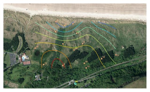
Figure 68: Piezometer locations and groundwater flow map, Winter 2021.
