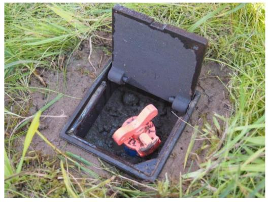
Figure 71: Completed Piezometer.
