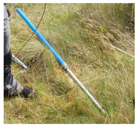
Figure 69: Hand installed Casagrande piezometer point.
