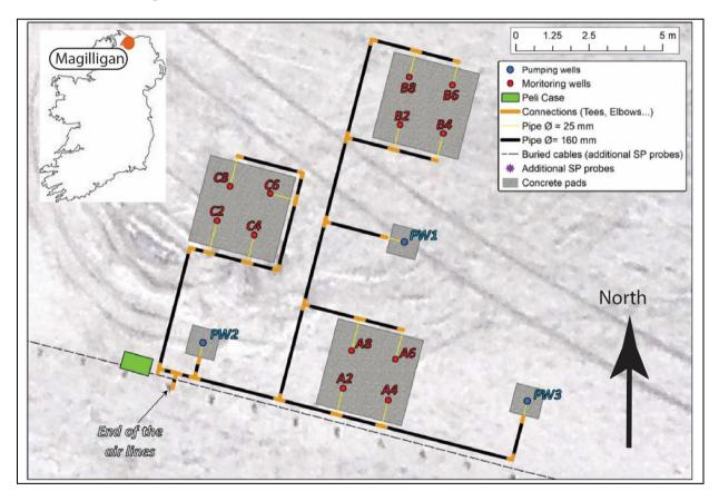
Figure 79: Location of Magilligan Test Site with positions of pumping and observation well clusters.
