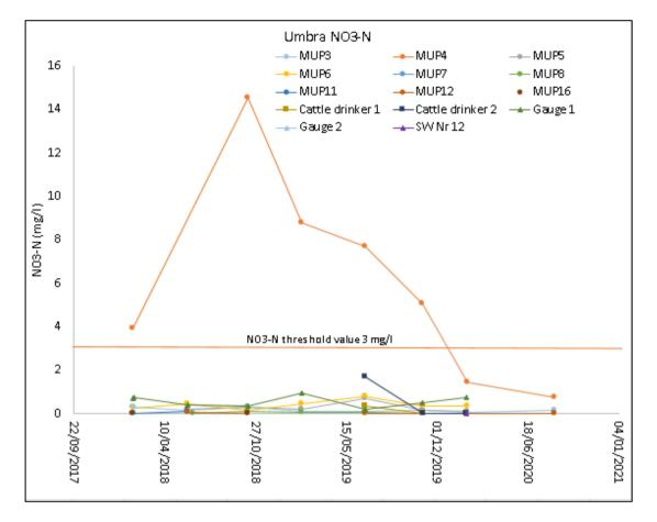
Figure 75: Groundwater NO3-N concentrations temporal changes.
