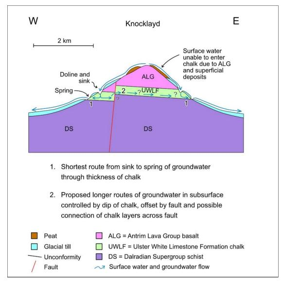
Figure 24: Schematic geological section through Knocklayd geology showing Karstic features and surface and groundwater flow (no vertical scale).
