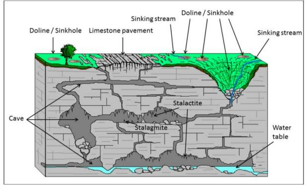
Figure 26: Schematic model showing Carboniferous limestone karstic features (from GSI website <u>https://www.gsi.ie/en-ie/programmes-and-</u>
