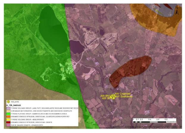
Figure 85: Bedrock Geology of the Lough Fea area (prepared by GSNI, 2021).
