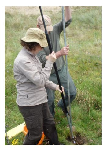
Figure 70: Piezometer Installation.
