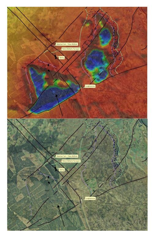
Figure 27A and B - Tellus Project magnetics with interpreted faults (black lines), base of Antrim Lava Group basalt (pink lines) and base of Ulster White Limestone Formation Chalk (green lines). Karstic features shown as points, and meltwater channel by black arrow.
