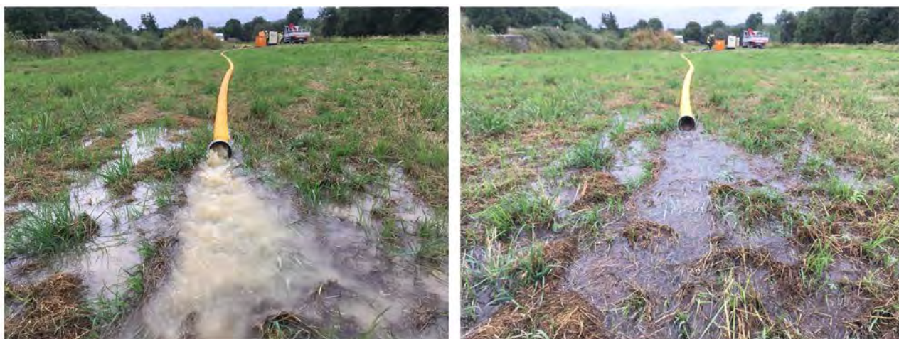
Figure 5: Turbid water at 47 m 3 /hr (left); sediment-free water at 21 m 3 /hr (right)
