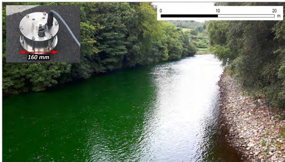
Figure 2 Fluorescein (FL) dye in the Avoca River upstream of White Bridge. Inset photo: GGUN-FL30 fluorimeter probe (courtesy of the Geological Survey Ireland).
