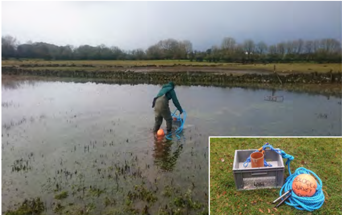
Fig. 2: Installing water level monitoring in Ballinturly turlough, Co. Roscommon (inset: logger housing)
