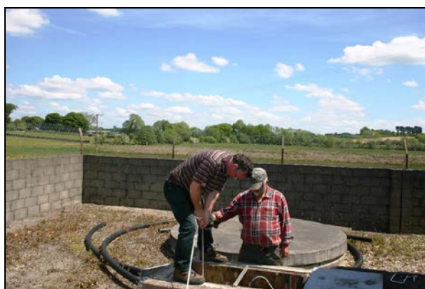
Image 2. Caherline Newtown GWS personnel dipping their borehole for water levels.
