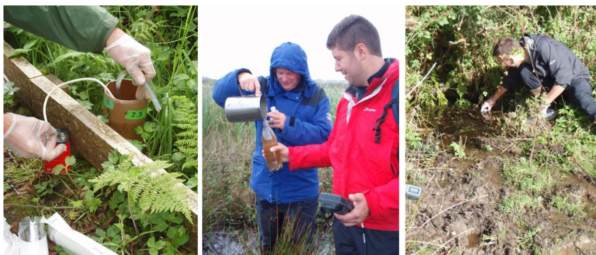
Figure 12 Left: an affordable 12v ‘caravan pump’ is lowered into a dipwell to obtain a sample. Middle: Les Colley and Adam Daniel use a stainless steel jug to collect water from a ditch Right: Jon Hudson collects a water quality sample from a diffuse seepage zone.
