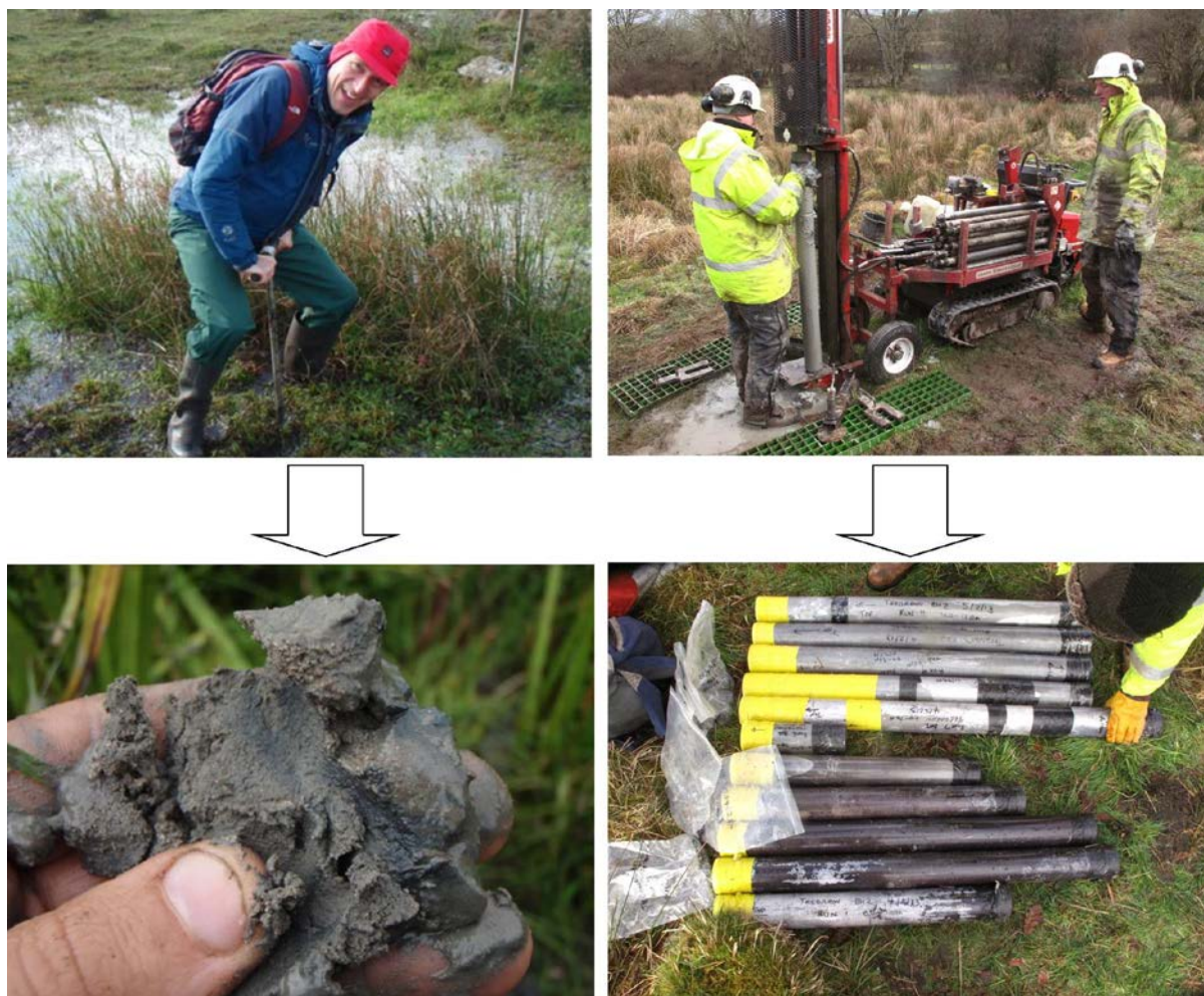
Figure 9 Left: Dr Mark Whitman (EA) uses a hand auger to collect information on the near surface deposits at Cors Geirch. Right: Stephen Thorpe (BGS) uses a Dando percussion drill to obtain an 18m core from Tregaron Bog.
